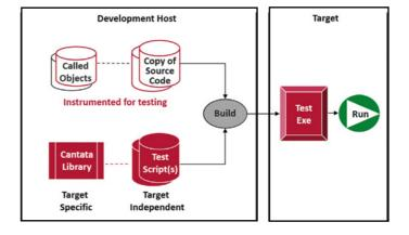
User code is driven by portable test scripts with target compatible libraries and built as a single test executable to run on multiple host or target platforms. Instrumentation is used for white-box access and code coverage, so production code is never modified for testing.
